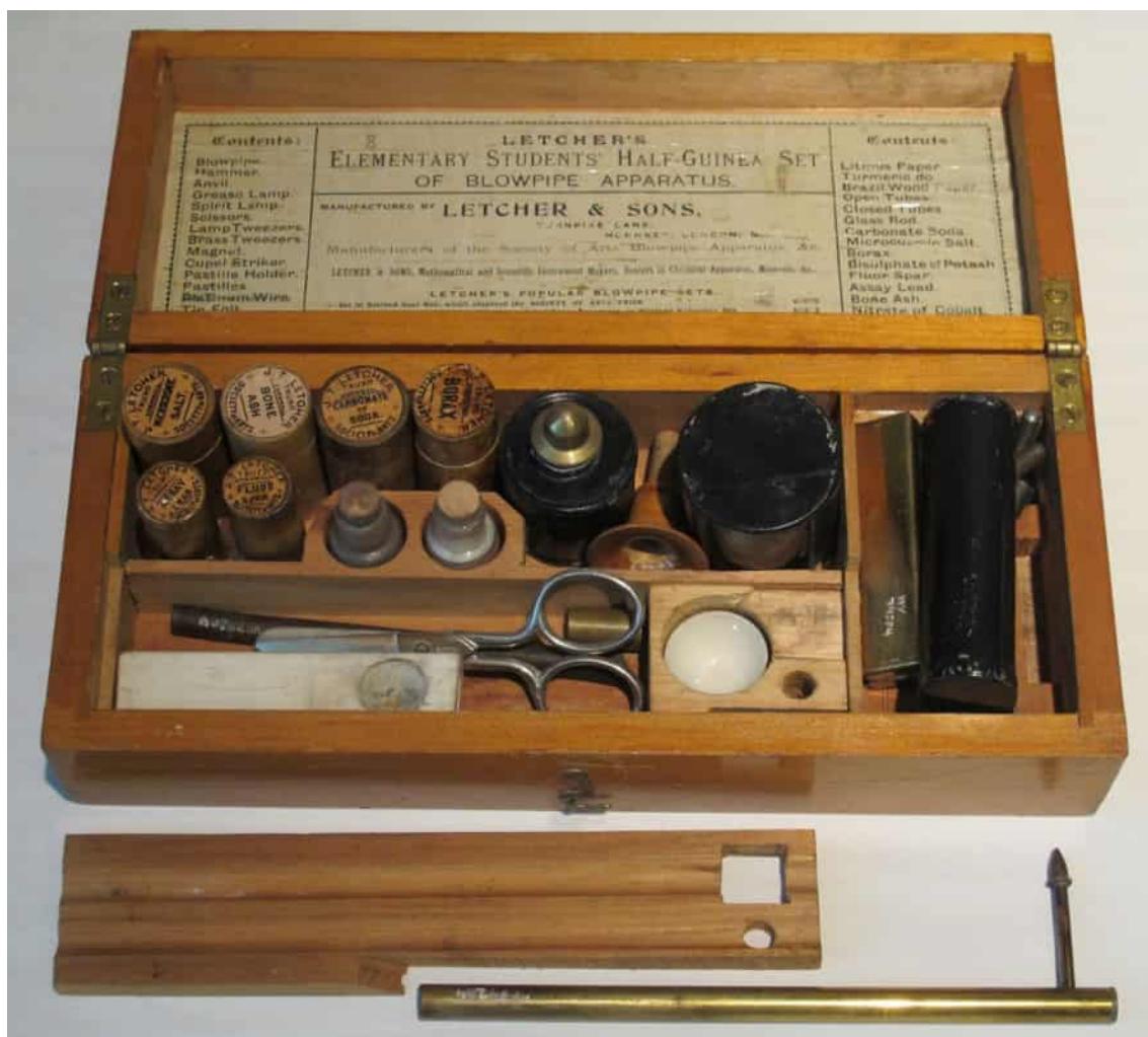
Blowpipe and related tools used by geologists. The blowpipe was used for quick mineralogical analyses in the field. Photo: Sanna-Mari Niemi, 2014.
