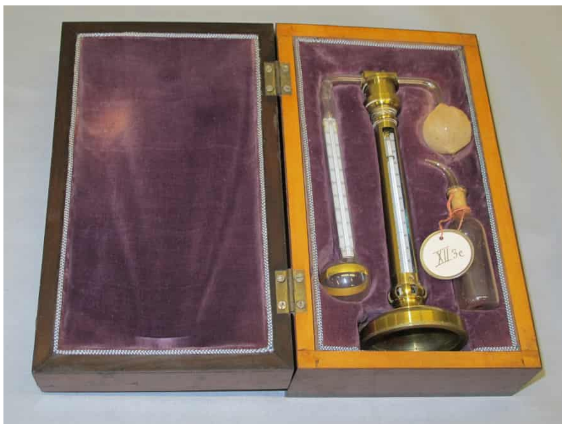
Daniell's condensation hygrometer, included in the cabinet of physics collection, from 1839. Photo: Susanna Åke, 2014.
