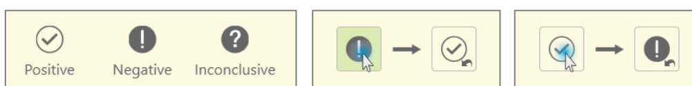
Figure 6: Quality Checks. Left panel: possible results. Center panel: overriding a negative quality check. Right panel: Overriding a positive quality check. Note the small arrow indicating an overridden quality check.
