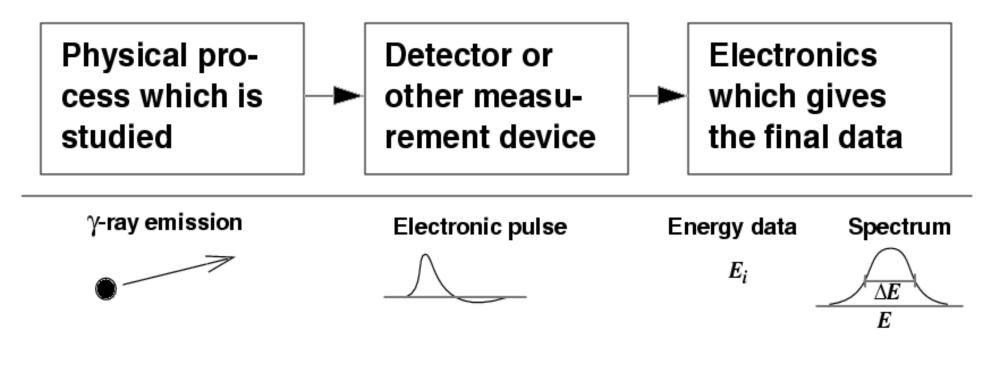
The latter two boxes represent the measurement electronics.
