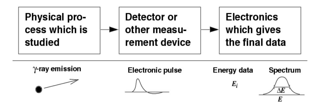
The latter two boxes represent the measurement electronics.
