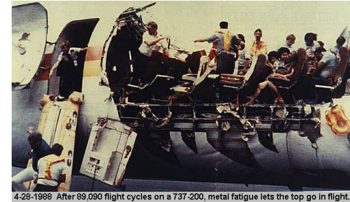
4-28-1988 After 89,090 flight cycles on a 737-200, metal fatigue lets the top go in flight.
