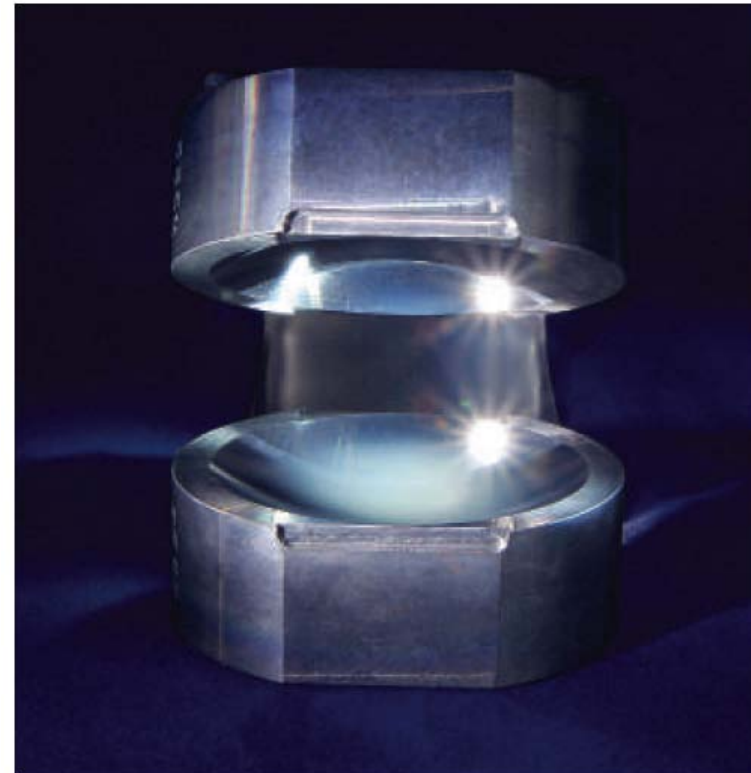
Figure 1 | They do it with mirrors. Gleyzes and colleagues' cavity for trapping photons 1 .
