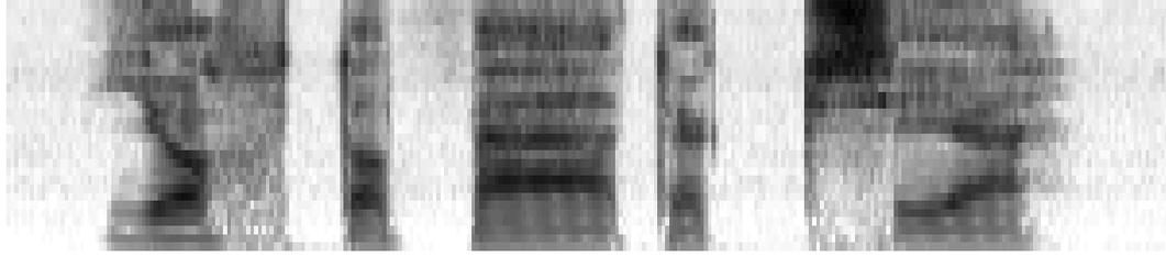
Figure 7.1: An example of the preprocessed spectrogram of a speech segment. Time increases from left to right and frequency from down to up. White areas correspond to low energy of the signal and dark areas to high energy. The word in the segment is “JOHTOPÄÄTÖKSIÄ”, meaning “conclusions”. Every letter in the written word corresponds to one phoneme in speech. The silent areas in the middle correspond to the consonants t, p, t and k, thus revealing the segmentation of the utterance into phonemes.
