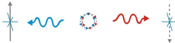
Figure 1. A decay process (at the center) outputs two photons (blue and red) which propagate in the opposite directions. As long as neither one of the two is subject to unequal forces, the polarization of one photon will remain intact relative to its mate but indetermined relative to any external frame of reference (an axis system in blue). The detection will place the polarization of one photon in the reference frame relative to the observer and the same frame will apply instantaneously also to the other photon provided that the correlated pair has remained unperturbed ever since it emerged from the decay.
