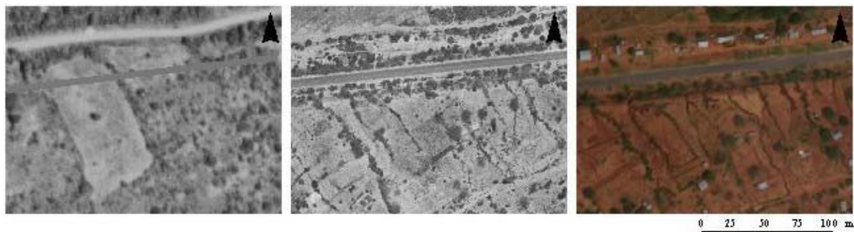
Figure 7. Rapid gully headcut propagation in Mwatate, as shown in aerial photographs in 1955 (left), 1993 (centre) and 2004 (right).
