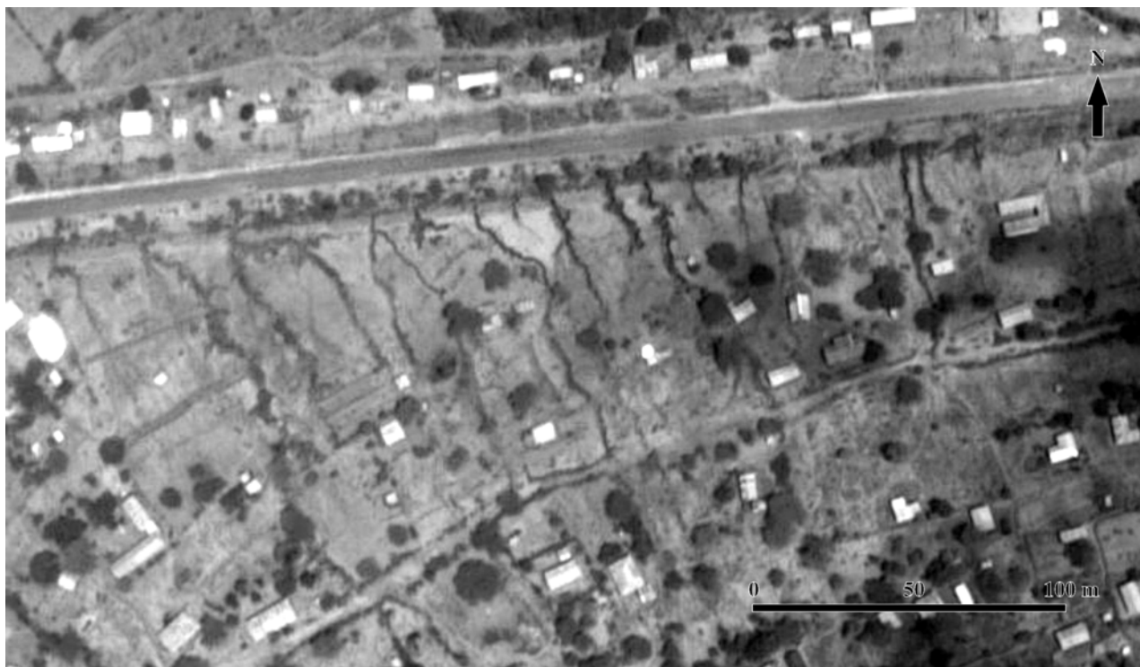
Figure 3. Gullies are extending to the squatters along the roadside in Mwatate. Aerial photograph orthomosaics (Photo from the year 2004, ground resolution app. 0.3 m) form the basis of the gully database of Taita Hills.
