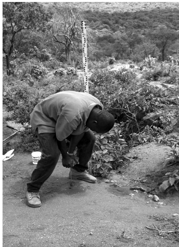
Figure 7. Shear vane tests were used both in field plots close to the gully head (above) and around the catchment areas. (Photo: Tommi Sirviö).
