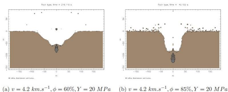
**Figure:** Comparison of crater profiles on highly porous surfaces (60 % and 85 %).
